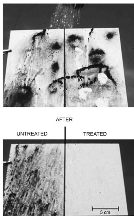
Figure 42. Soot-coated Formica plates. The left plate in each image is an untreated surface that shows no lotus-effect self-cleaning thus soot removal is inefficient. The right plate in each image is coated with micro-powdered PTFE to give a super-hydrophobic surface from which soot is easily removed with water. Reproduced with permission from ref. [122].
